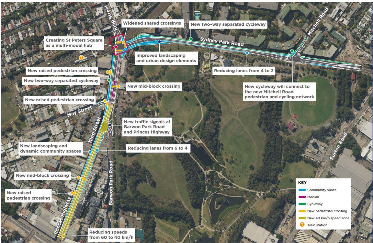
Figure 1: Plan showing the proposed changes to Sydney Park Road, King Street and Princes Highway (Source: Transport for NSW)
