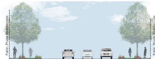
Figure 2: A diagram showing a desirable allocation of road space on New South Head Road (Source: Woollahra Council)
