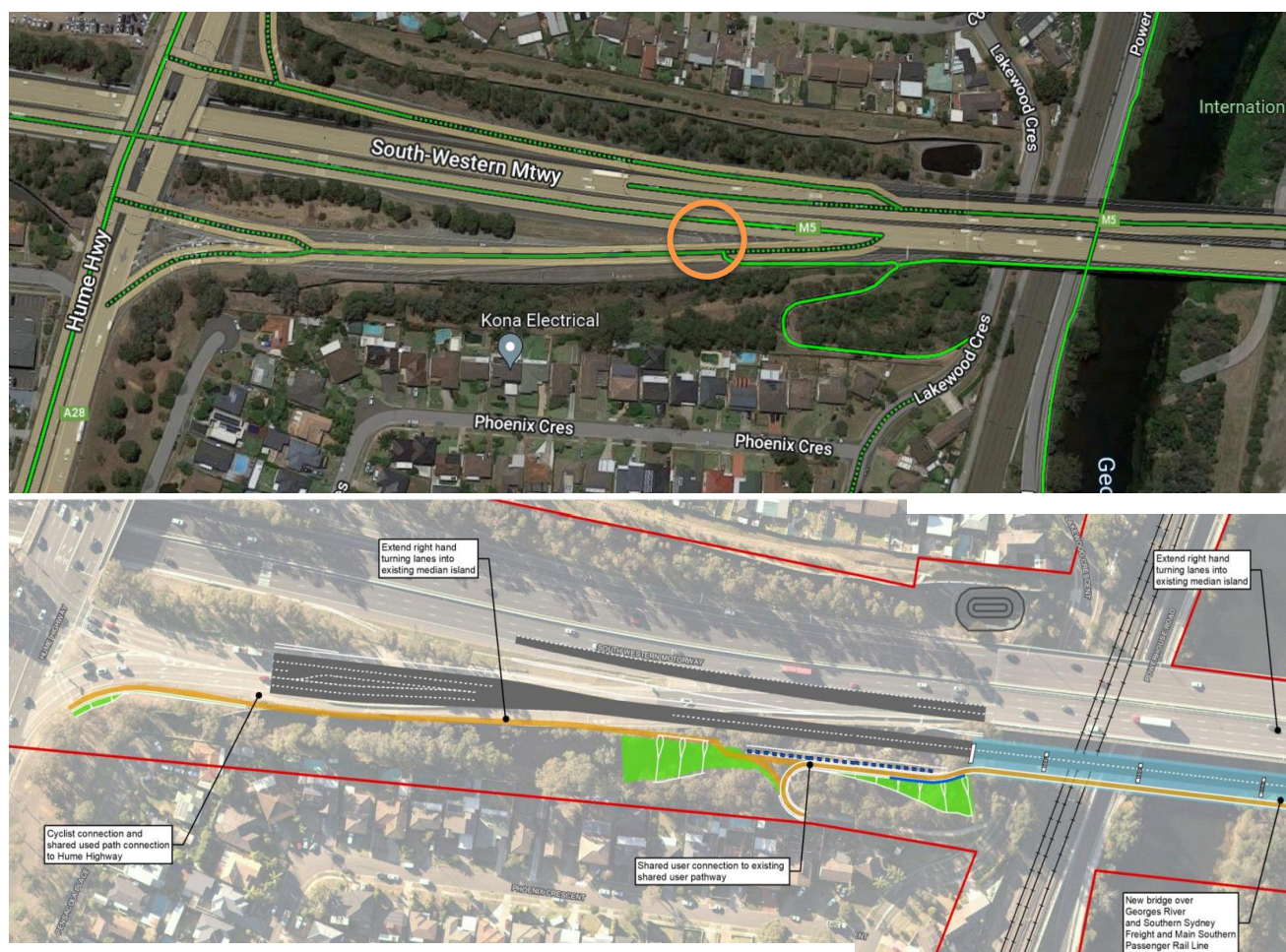
Figure 9: Access to the motorway heading west from the shared path from Lakewood Crescent is currently possible by crossing the slip lane at the point marked by an orange circle. It appears that this connection will no longer be possible. (Source: Google Maps / TfNSW, 2022 REF)
