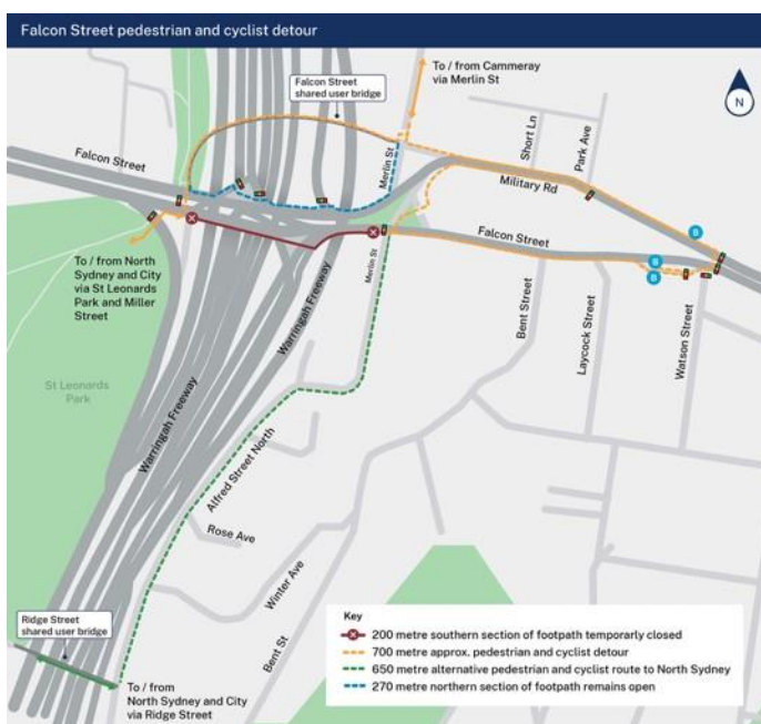
Figure 3: Without a shared path on the southern side of the freeway bridge, or an underpass or new signalised surface crossings on the eastern side, pedestrians must back track to Watsons Street to cross from Merlin St to St Leonards park, adding 500m to the walk. This is the current situation as indicated on the detour map but it is not acceptable in the long term. (Source: TfNSW)
