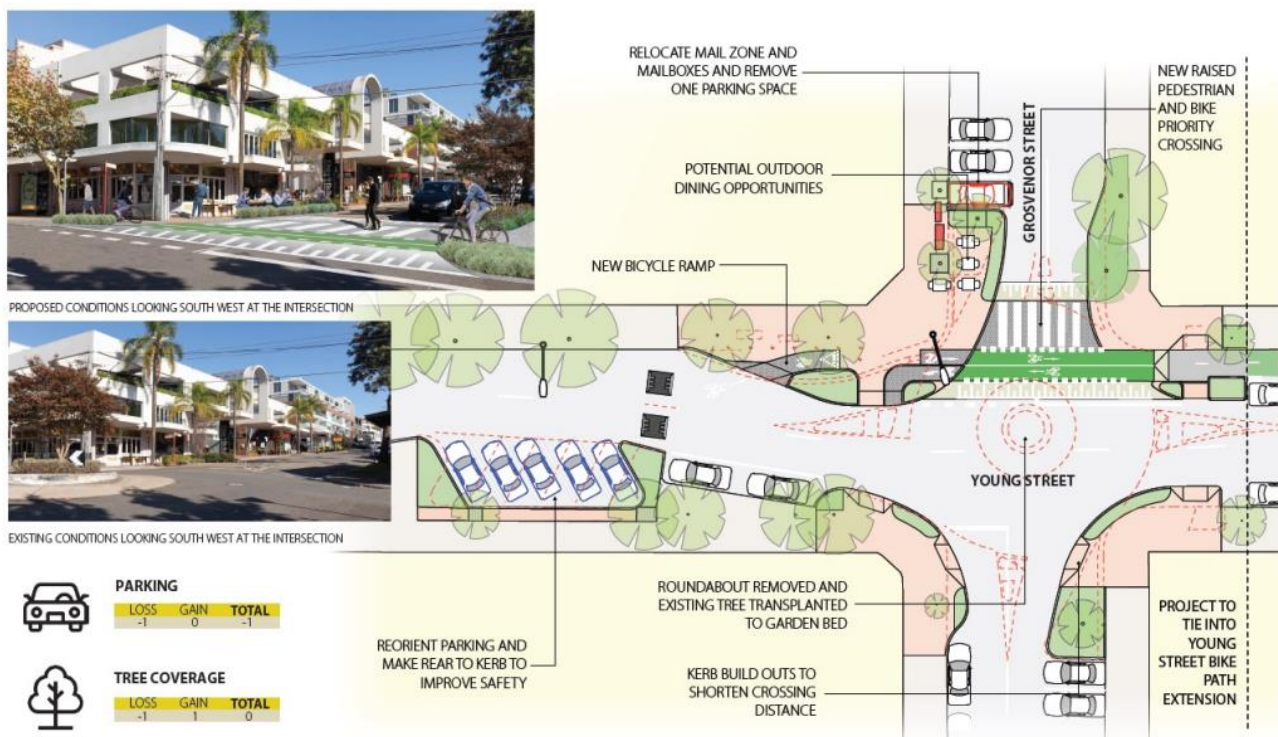
Figure 2: The plans for reconfiguring the intersection of Young Street with Grosvenor Street (Source: North Sydney Council)
