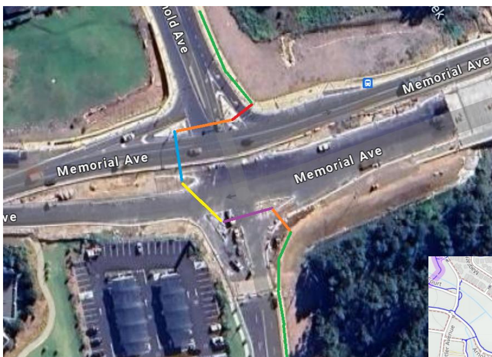
Figure 1: The inset plan shows the gap in the path network that the shared paths delivered by the Memorial Avenue project will fill. However, the missing crossing on the eastern side will force path users travelling from north to south to cross six road sections (main image). Note that there Kellyville Grove Shopping Centre in the south west corner is a key local destination but access from bus stops will very difficult. (Images: Open Street Map / Google Maps / CAMWEST)
