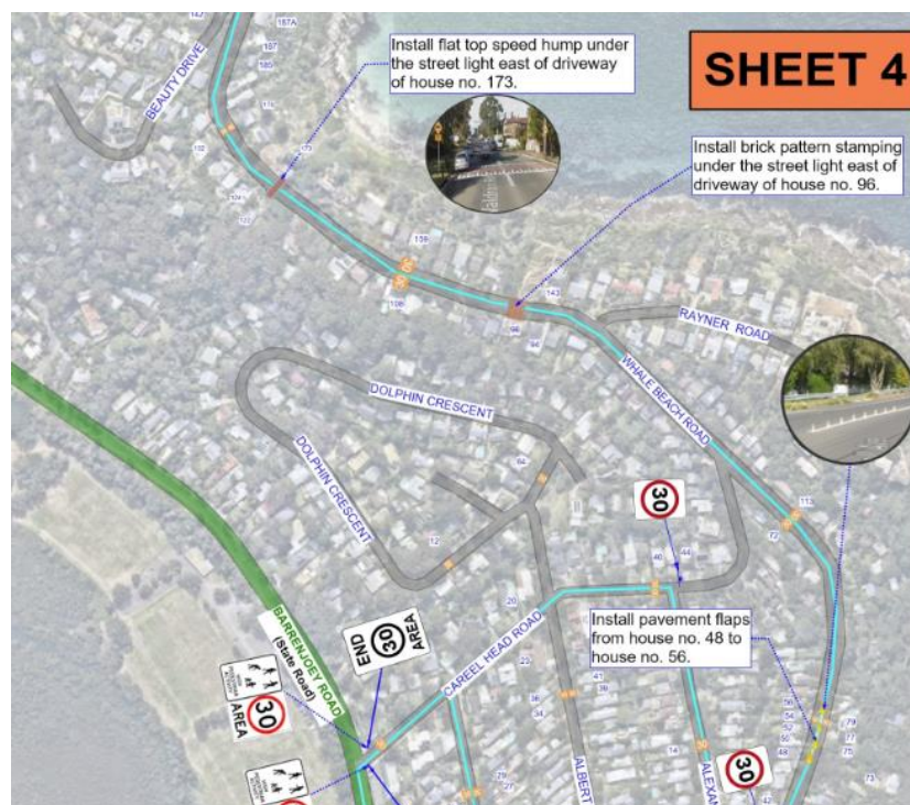
Figure 1: Extract from the plans for Avalon Beach to Palm Beach shows the tiny images used to explain what is meant by 'pavement flaps' and 'flat top speed humps'. (Source: Northern Beaches Council)
